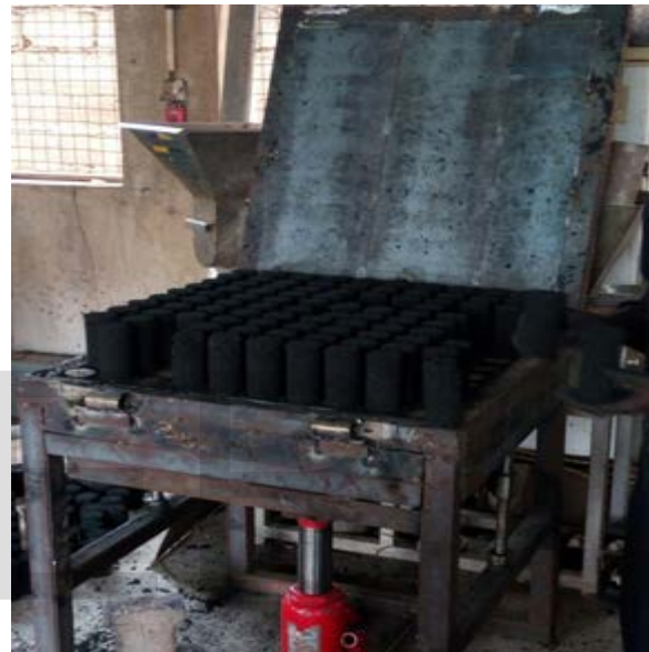
Ejected briquettes on the hydraulic briquette press
